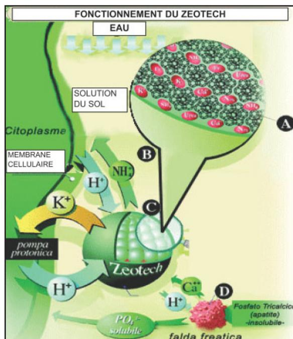
**A** - ZEOTECH 300 EST DE CHARGE NEGATIVE. II ABSORBE LES CATIONS NH<sub>4</sub> - K + & Mg
